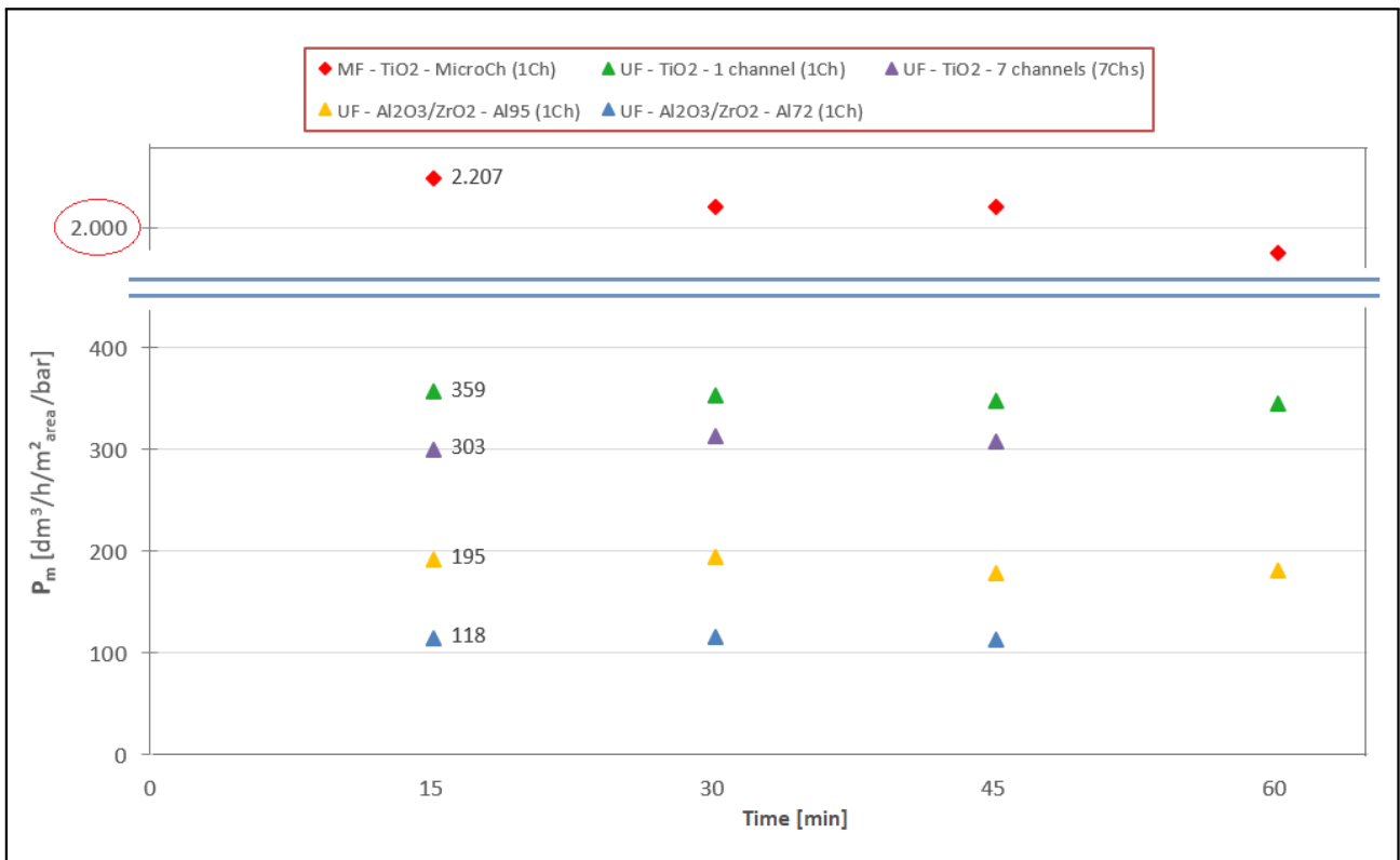
Figure 4.1: Changes of membrane permeability during UF (100kDa) and MF (0,2 \mu m) of pure water through Al 2 O 3 /ZrO 2 (1 channel) and TiO 2 (1 and 7 channels) ceramic membranes (process parameters : TMP = 3 bar, CFV = 3 m/s)
