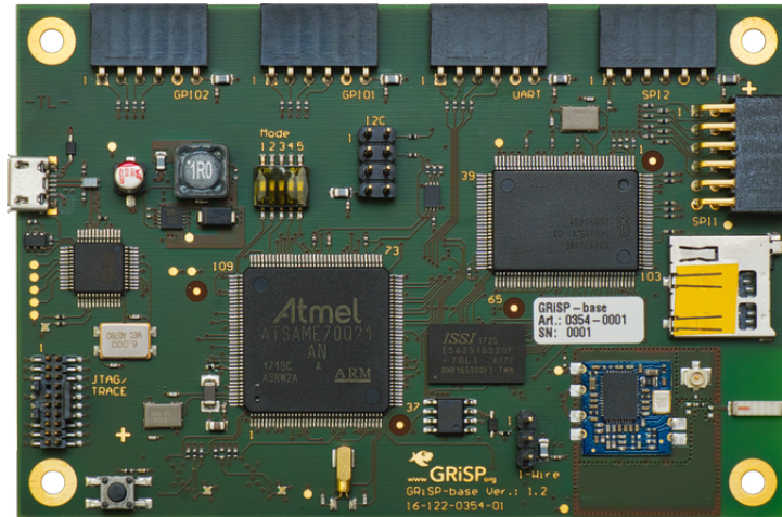
Figure 3.: GRiSP board - Image was taken from https://www.kickstarter.com/projects/peerstritzinger/grisp-2
