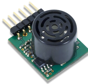
Figure 4.: Pmod MAXSONAR: Maxbotix Ultrasonic Range Finder.
