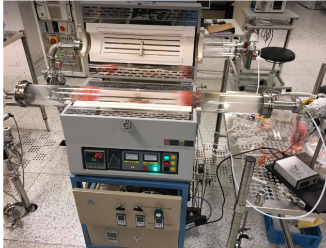
Figure 3.1: Chemical Vapor Deposition (CVD) device used for the fabrication of the sample.
