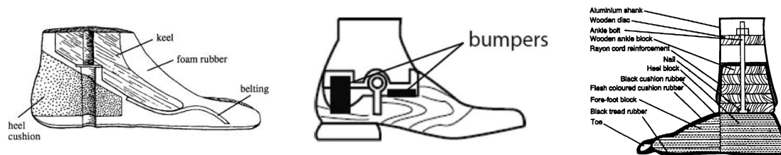
Figure 2.8: Sketches of conventional feet. (left) The SACH foot [18], (middle) The Uniaxial foot [13], (right) The Jaipur foot [19]
