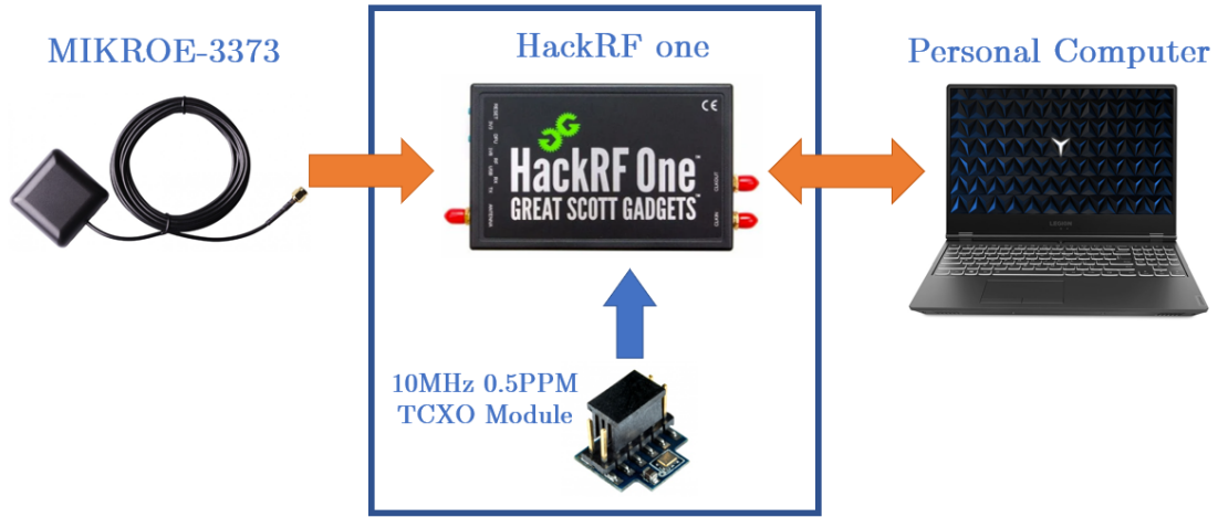
Figure 6.1: GNSS data capture setup
