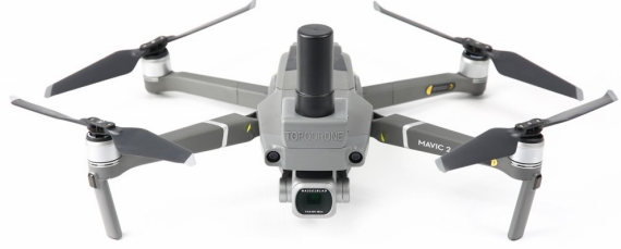
(b) Picture of the Mavic DJI Pro 2 modified with an antenna (black cylinder). Source: Topodrone
