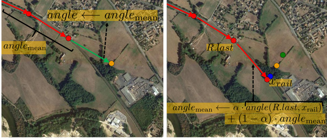
(a) At the start of the iteration x , angle_{mean} is based on the angles between last points in red. It is used to estimate the next point in orange.
