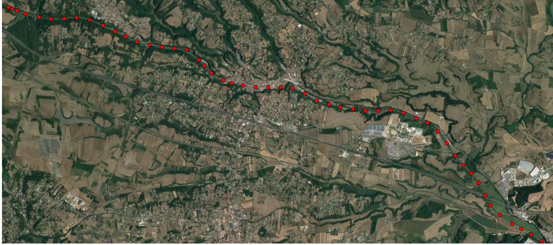
Figure 8.12: Sample of the outputs of the rail tracking algorithm
