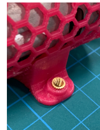
Figure 3.5: Picture of a positioned threaded insert on the motor casing.
