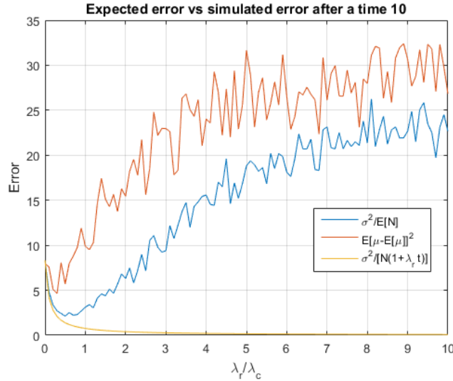
Figure 2.8: Comparison of the effective mean square error of the estimation, the definition of the bound on the error based on the simulation, and the lower bound defined by the number of agents that went in the system.
