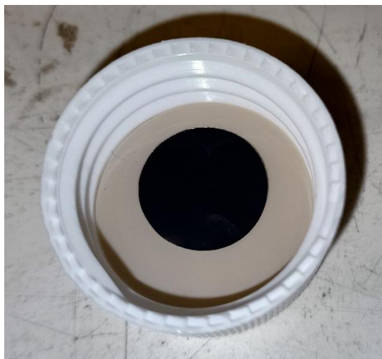
Figure 3.7: LFP cathode prepared by NMP based slurry method, Ø 13 mm.
