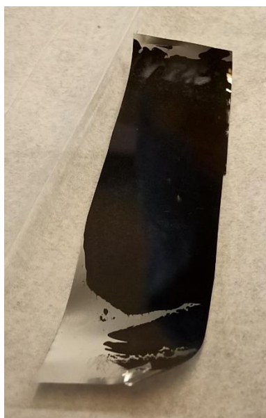
Figure 3.8: Aluminium foil with coated slurry for hybrid cathode (before heating).
