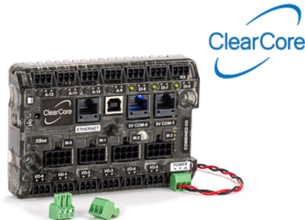
Figure 6.5: Clearcore - industrial I/O and motion controller made by TEKNIC
