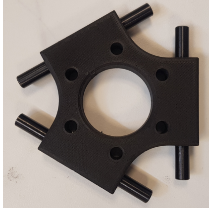
Figure 7.3: End effector 3D printed with the MAKEFORGED printer with Kevlar layers.
