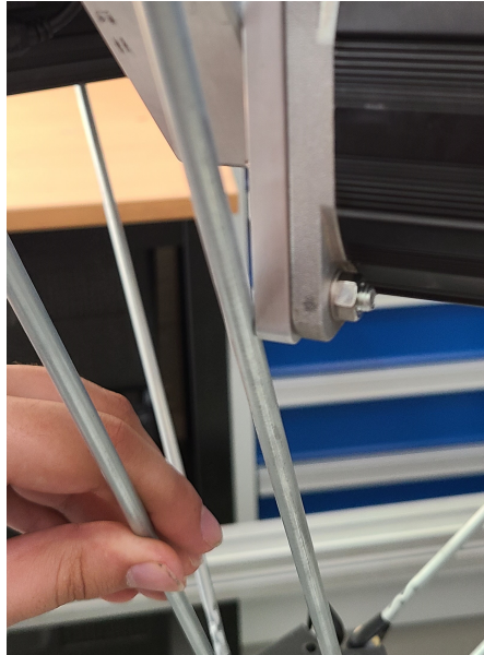
Figure 7.5: Collision between the distal arm and the motor mounting bracket.
