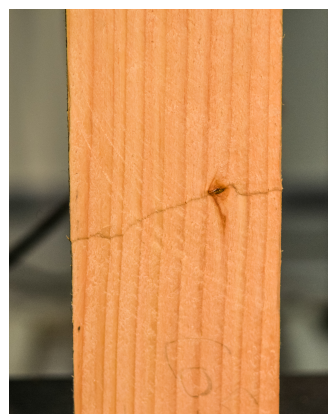
FIGURE 9.10 – Rupture type en compression
